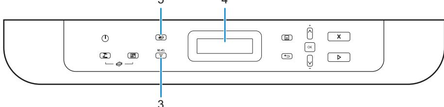
**3 "W" (Wi-Fi) button (Dell Multifunction Printer | E514dw and Dell Multifunction Printer | E515dw only)**
