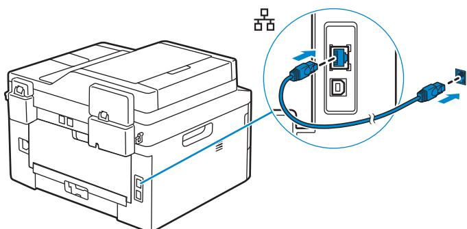
**For fax connection, connect telephone line cable (Dell Multifunction Printer | E515dn and Dell Multifunction Printer | E515dw only)**
